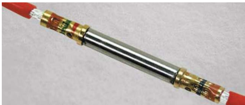
An example of a good crimp showing the exposed wire
