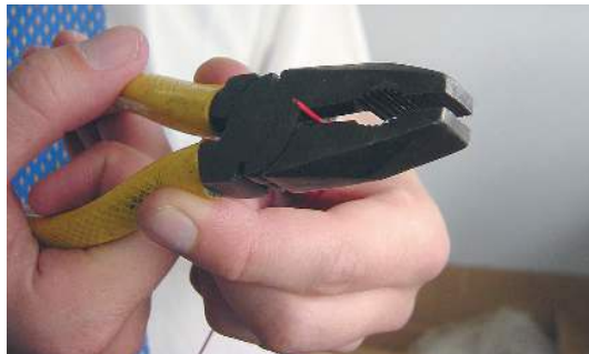
Not the best way to strip insulation. Pliers may remove the insulation, but are also likely to break and remove strands of the wire too.
