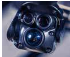
Integrated camera NextVision DragonEye2 optical / thermal camera
