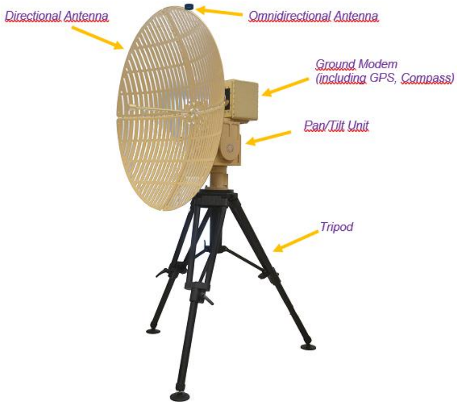
Figure 4. Ground Data Terminal Assembly
