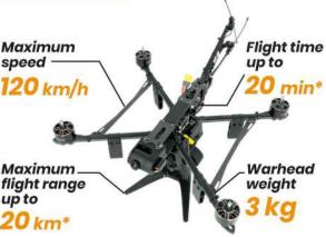
The drone is equipped with a 6s3p or 6s4p battery and a payload release system.
