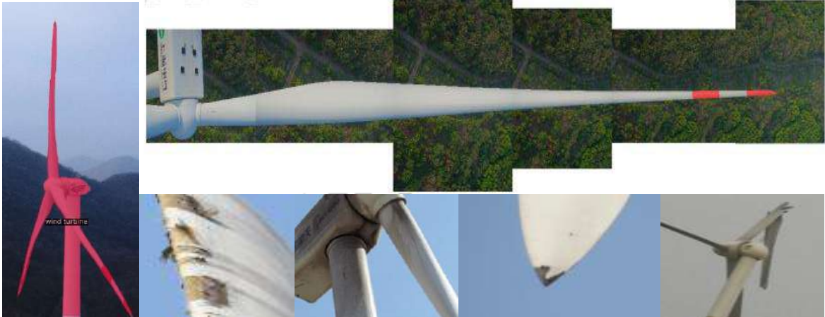
Wind inspection AI automatically recognizes the orientation of the wind turbine, and multiple captured images can be automatically spliced into complete wind turbine blades. The platform AI intelligently analyzes various types of defects in the wind turbine
