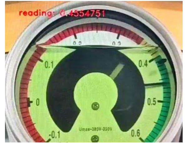
AI intelligent reading of device meter pointers
