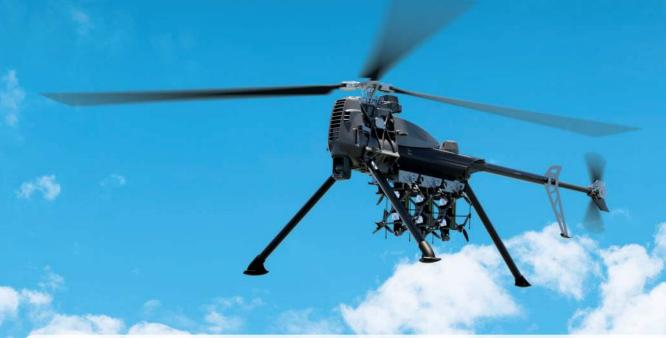
The TALON DT-150 is a very compact Group 2 unmanned aerial system (UAS) developed as a smaller counterpart to the TALON DT-300. Designed for versatility and portability, the DT-150 serves various applications, including reconnaissance, surveillance, and target acquisition as well as the ability to deliver useful logistics or support with up to three FPV drones.
