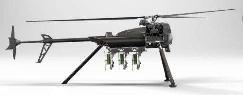
THE DT-150 CAN BE EQUIPPED WITH UP TO 3 DRONES OR ALTERNATIVELY CARRY UP TO 22.5KG OF CARGO BAGS
