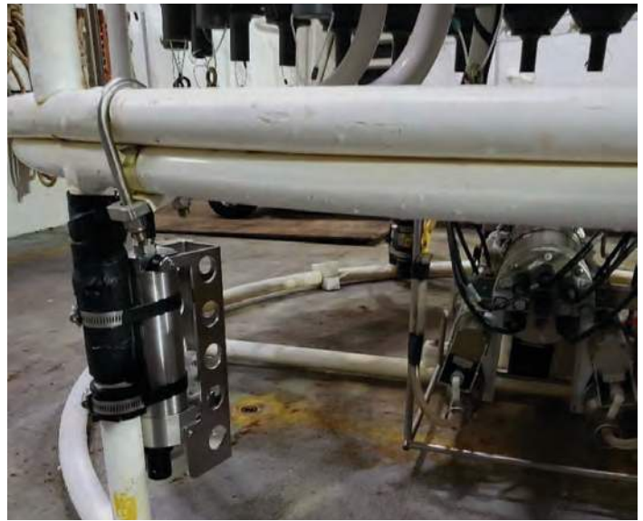
D2 CTD on R/V Endeavor Rosette (4m, 5-pin CTD cable used)
