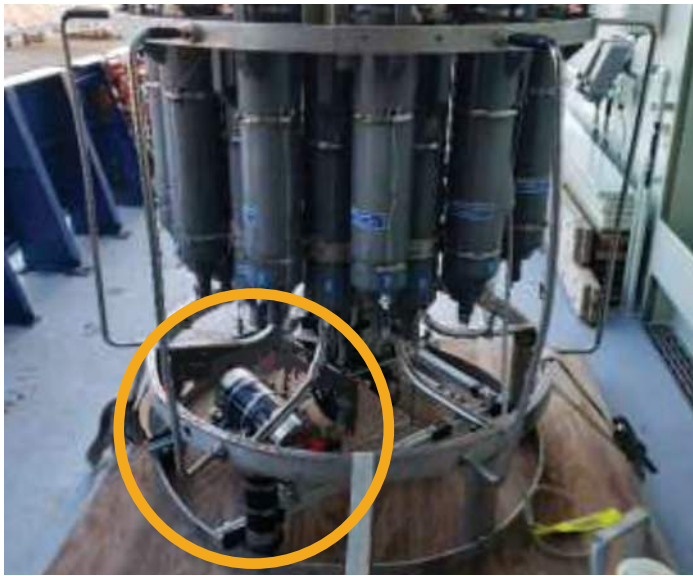
D2 CTD and WHOI Data Logger on Water Sampler Rosette
