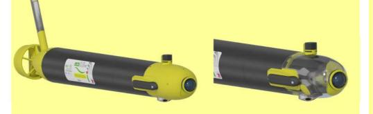
Payload: NBOSI CT • Marine Sonic Technologies Scout ARC Mk II Side Scan Sonar (900, 1200, 1800kHz or dual frequency) • ecoCAM 4K camera • Nvidia Jetson Orin Nano Backseat GPU • Nortek Nucleus DVL-1000 (with currents) • Nano-modem (option for Sonardyne AvTrak6)
