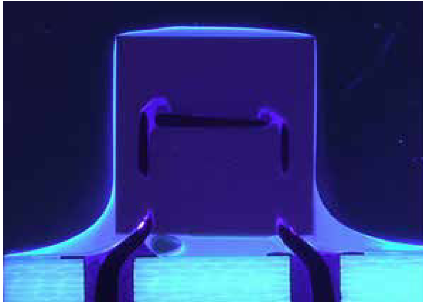
SEM image of conventional conformal coating coverage (Source: IPC-SMTA)
