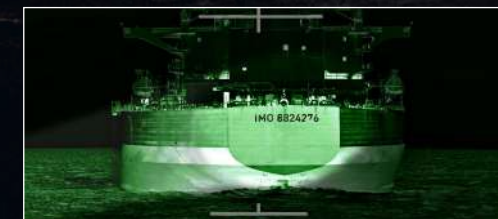
Covert IR Filter - read ships registration at night
