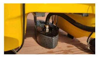
**Wassp S3** is one of the world's most cost-effective, professional survey and mapping multibeam sonar solutions. Designed as a mid-level sounder, the S3 will meet your budget, operational needs and future technology roll-out. And it lets you cover your survey area up to 10 times faster than a single-beam sounder. It can be integrated in SEABOTS's SB 100 PRO USV and it's compatible with HYPACK, BeamworX, EIVA and QINSy and others with a range of export options.
