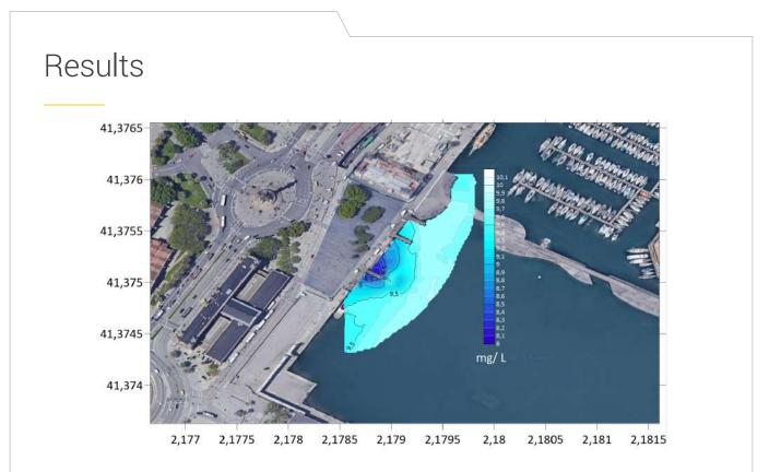
Oxygen concentration measurated by a WIMO Multiparametrical probe integrated on the SB 100 PRO.
