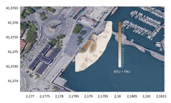
Turbidity measurated by WIMO Multiparametrical probe integrated on the SB 100 PRO.
