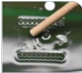
Figure 2. Control (5 minutes after cure) Adhesive under component was completely wet
