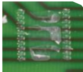
Figure 5. Day 3 at RT Adhesive under the component was soft with a waxy surface.
