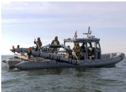
Sailors from Mobile Diving and Salvage Unit (MDSU) two launch the MK18 underwater unmanned vehicle (UUV) during a training evolution at Joint Expeditionary Base Little Creek-Fort Story. (U.S. Navy photo by Mass Communication Specialist 2nd Class Benjamin Woody/Released)
