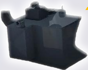
Main auxiliary fuel tank with 13 liters.
