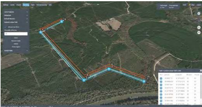
Image 5: Planning the aerial survey of a linear object in the xGroundControl station at a strip width of 50 m (164 ft).
