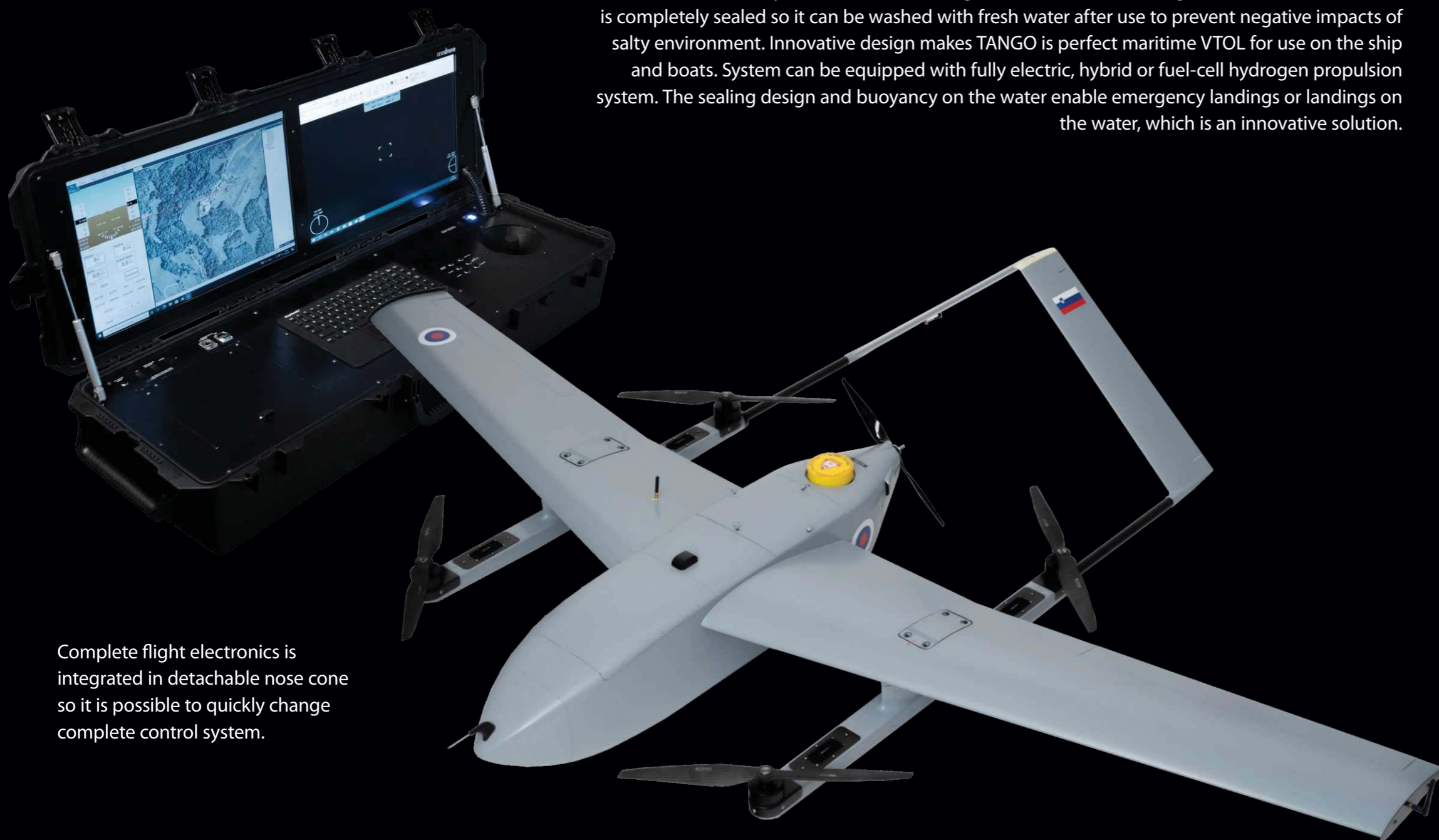
Extremely large cargo space dimensions (45x23x23cm) allow to install a gimbal of large dimensions with different characteristics.
