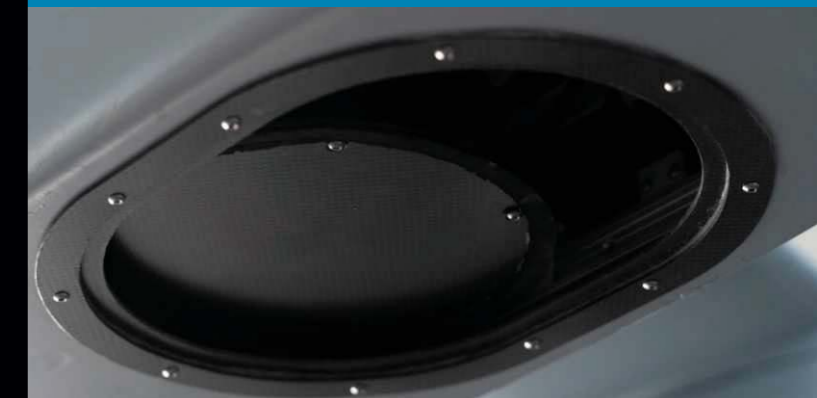
TANGO fuselage is completely sealed for maritime use.
