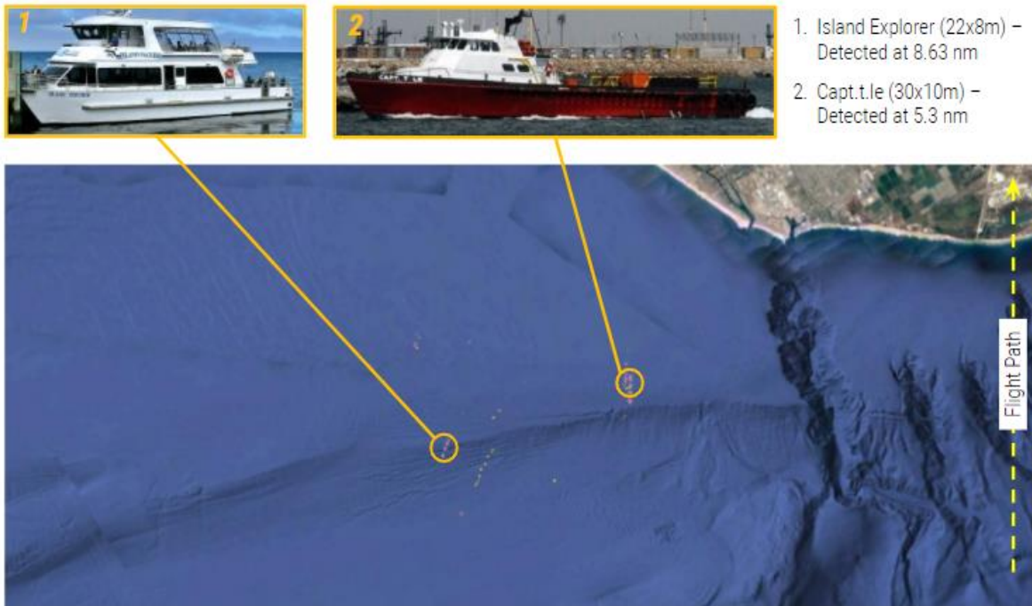
Figure 8: (Top) Detection and Tracking of Vessels, with AIS Data to Corroborate. MMTI mode uses Doppler to automatically search for, detect, and track moving targets and other objects in maritime and littoral environments. MMTI can be used to perform a focused search by commanding the radar to continuously monitor a preselected area of interest, or perform a wide-area search in which the radar uses a scan pattern to search a wide area. NOTE: The targets depicted in this diagram were targets of opportunity, and the detection ranges do not represent the maximum ranges of IMSAR radar system capabilities.
