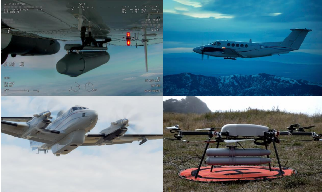
Figure 3: Successful Integrations of IMSAR's Family of Low-SWaP-C Radar Systems. IMSAR has successfully increased the ISR capabilities of multiple aircraft, including (from upper left to lower right) the King Air C90, the King Air B200, the King Air 350, and the Skyfront Perimeter 8.
