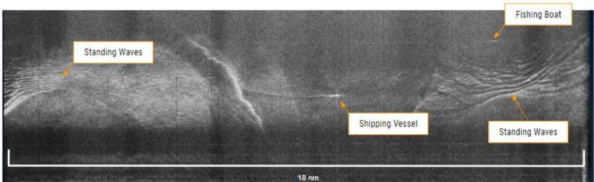
Figure 9: Actual SAR Ocean Imagery from an IMSAR Radar System. This image shows the radar’s ability to produce real-time high resolution SAR imagery products useful for detecting and locating surface vessels in the scene.
