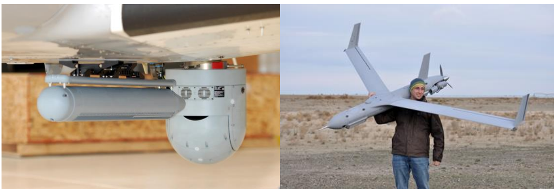
Figure 4: IMSAR's NSP-7 Radar System Integrated with an Optical Sensor (left) and the NSP-3 radar system components deeply integrated into the ScanEagle UAS platform (right)
