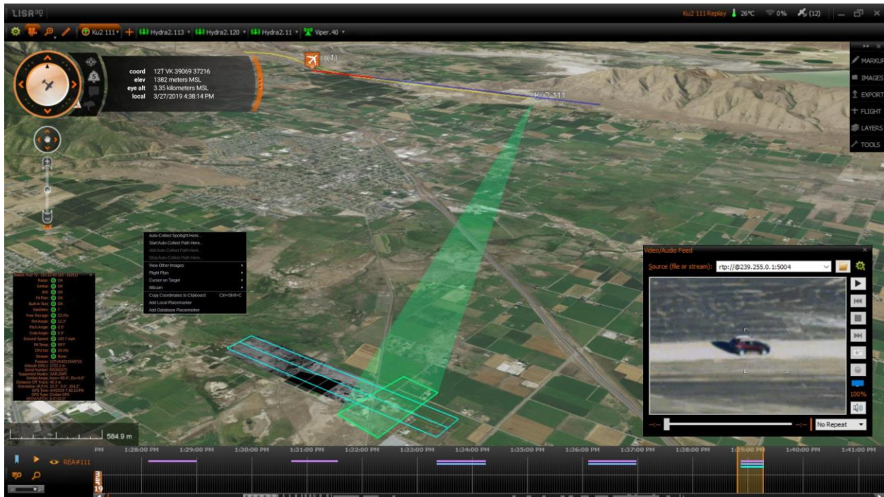
Figure 10: Lisa3D C2 and PED User-Interface. In Lisa 3D, sensor data can be overlaid on an existing 3D optical map or represented with icons to make data easy to understand. Operators can annotate and mark sensor data, and Lisa 3D will automatically highlight the annotations and marks on the map, timeline, and calendar.
