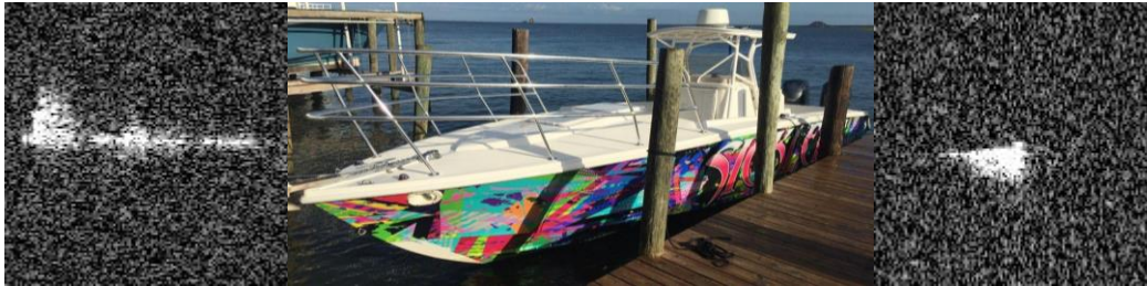
Figure 5: ISAR Data from Maritime Collection with the NSP-7. These ISAR images (left: 0.1m resolution) and (right: 0.3m resolution) were taken of the craft pictured in the center, with the following specifications: 10,000' AGL, 25-degree depression/grazing angle, 4 mile standoff range, sunny conditions.
