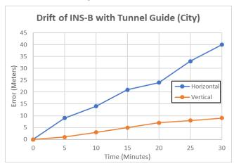
The average drift rate of the second sample set was calculated to be 0.2% DT over the course of the 30-minute outage with a peak drift of approximately 45 meters. These results show that **Tunnel Guide** significantly improves performance accuracy during GNSS outages, at a much lower cost.
