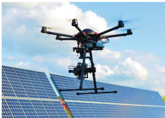
Figure 1: Drone with Raptor 640 SWIR camera
