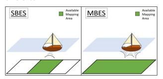
With ping rates of MBESs as high as 50 Hz, you can be confident that regardless of the water depth, when it is paired with an Inertial Labs MRU-PD, acceptable surveying data can be gathered without having to perform numerous passes. The MRU-PD has been tested and works seamlessly with MBES manufacturers like: Teledyne, Klein Marine Systems, Kongsberg, ITER SYSTEMS and NORBIT.
