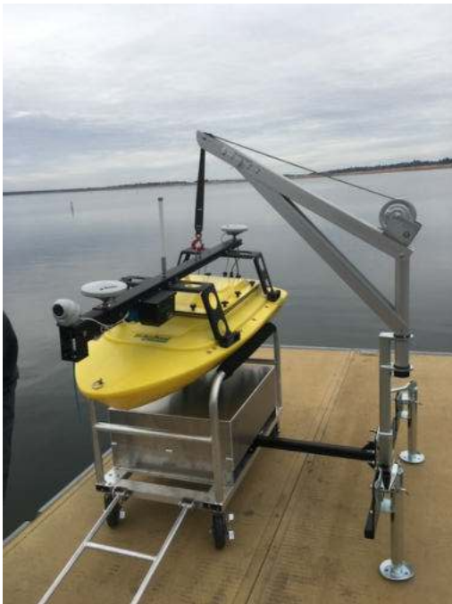
EchoBoat with EchoCart and Launch and Recovery davit system to lower off a dock or wall.
