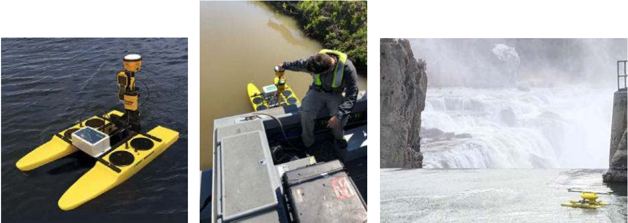
HyDrone-G2, L to R: with AutoNav, Seafloor Systems HydroLite-TM™ echosounder, Trimble SPS985, and TSC3 data logger running SCS900. USGS using with Teledyne RDI RiverPro. Shoshone falls, with integrated PicoMB Multibeam sonar
