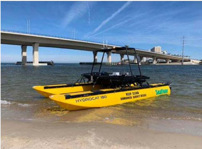
HydroCat-180 with IDH SeaBat T50, INS Type 30 (Hampton Roads Tunnel Connectors)
