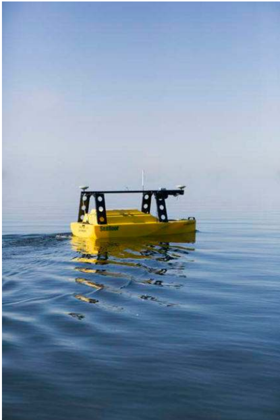
EchoBoat-240 with SeaBat T50 integrated on it.
