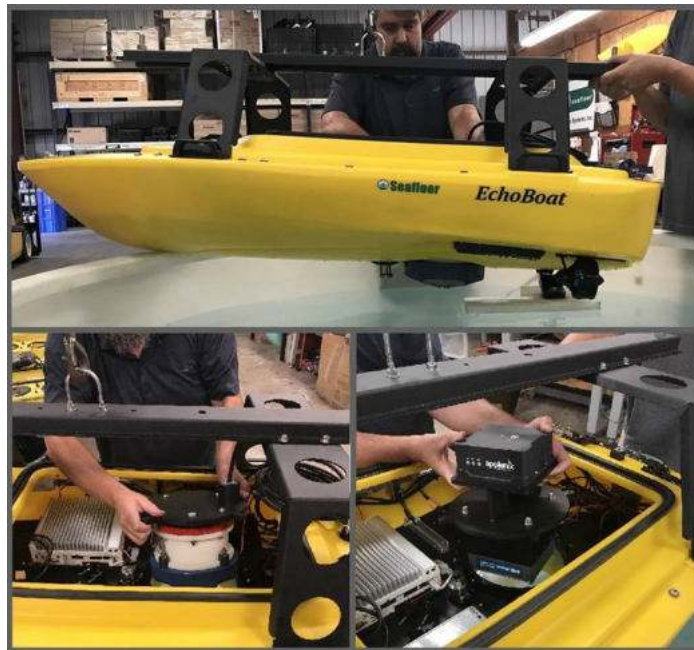
Swapping a Multibeam sonar and ADCP system in/out of the thru-hull moonpool.
