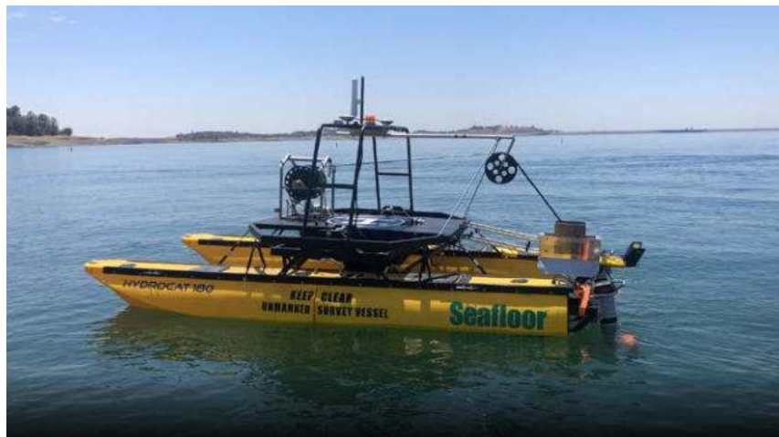
HydroCat-180 with a Winch towing a Klein MA-X View 600 sidescan sonar
