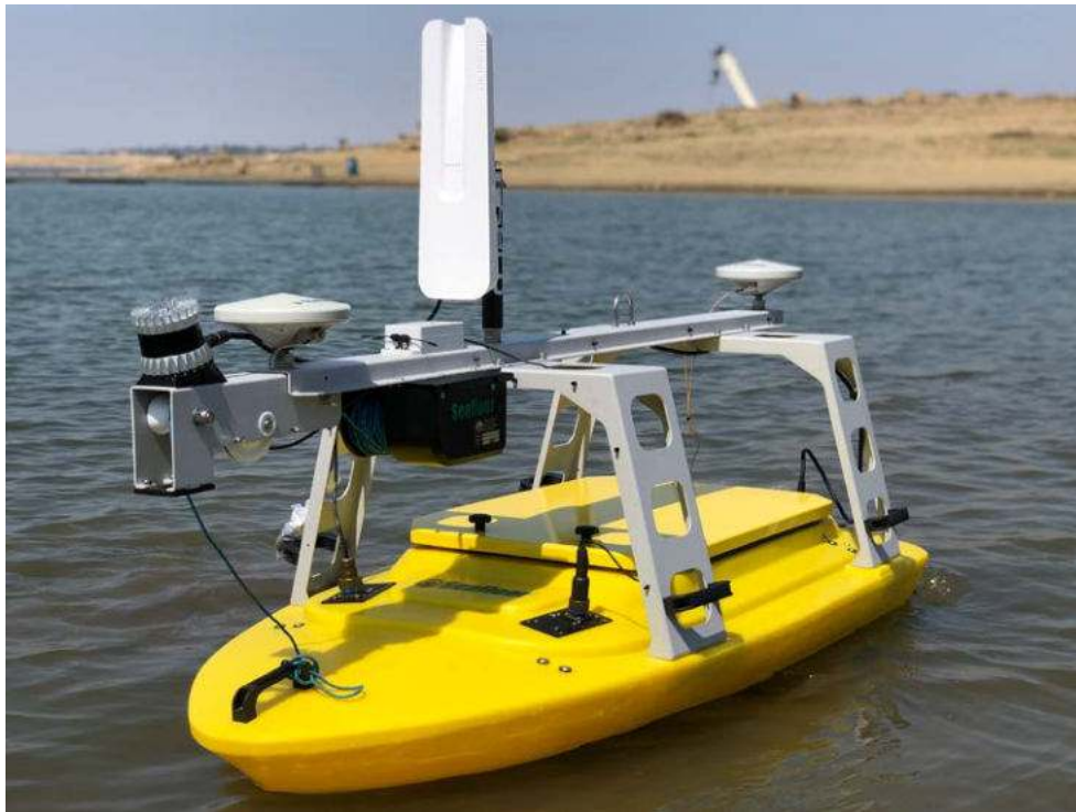
EchoBoat-160 with integrated Multibeam sonar, Inertial Navigation System, Sound velocity sensor, Sound velocity Profiler, LIDAR scanner, and onboard PC with hydrographic data collection software
