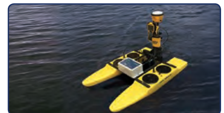
HyDrone™ ASV with Trimble SPS 585 and TSC3
