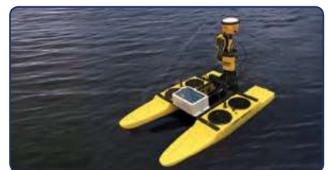
HyDrone™ ASV with Trimble SPS 585 and TSC3
