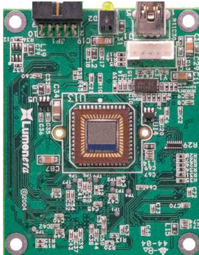
Figure 1.2: Teledyne Lumenera board level camera without the optical window (–WOG)
