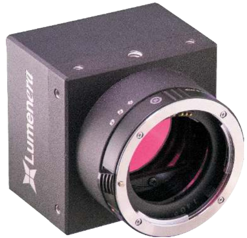
Figure 3.1: –WIR option on the optical window of a Teledyne Lumenera Lt29056H camera
