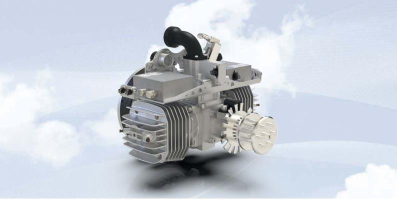
The 2-cylinder engines of the SP-170 series are designed with twin spark plugs and can be equipped with a carburetor or a fuel injection. The generator is mounted on the rear output shaft. All engines are equipped with the ignition HKZ215 and the ECU030. The electronics of the HKZ215 can be installed on an additional system carrier which sits on top of the cylinders. The engine is available with or without system carrier.
