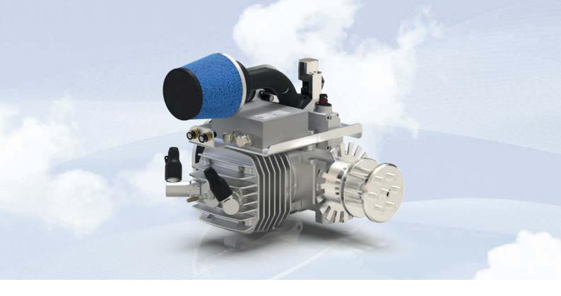
The single cylinder engine of the SP-55 series is designed with twin spark plugs and can be equipped with a carburetor or a fuel injection. The rear output shaft and the position of the carburetor or the fuel injection on the side, make this engine to one of the most compact 1-cylinder engines on the market. Because of the rear output shaft, a generator can be mounted on the back of the engine. All engines are equipped with the ignition HKZ215 and the ECU030.
