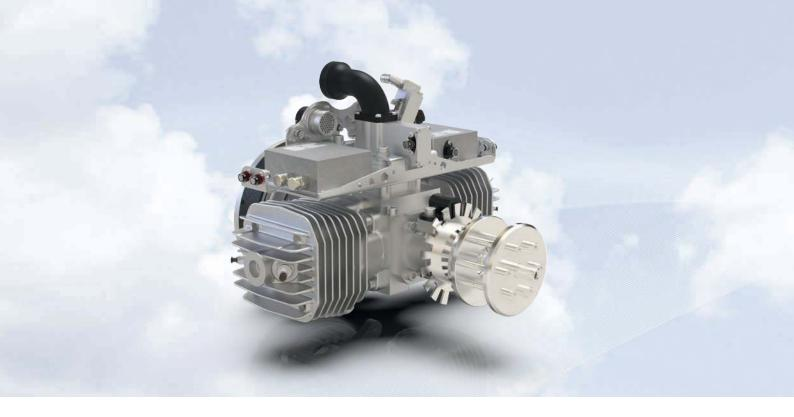
The SP-210 series is designed with twin spark plugs and can be equipped with a carburetor or a fuel injection. The generator is mounted on the rear output shaft. All engines are equipped with the ignition HKZ215 and the ECU030. The electronics of the HKZ215 can be installed on an additional system carrier which sits on top of the cylinders. The engine is available with or without system carrier.
