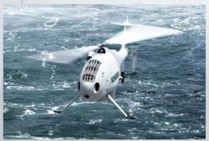
It is fully marinized against corrosion through the extensive use of carbon fibre composite materials, stainless steel, titanium, anodization and special coatings.
