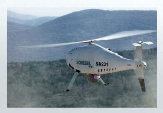
The S-100 is the master of complex terrain where no airfields or runways exist. Furthermore, as a VTOL system, it needs no prepared area or supporting launch or recovery equipment.
