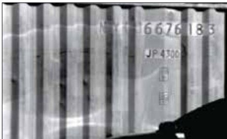
Paint penetration reveals underlying features
