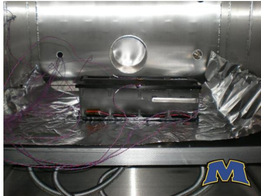
Figure 7: final vibration and thermal vacuum testing, Courtesy of Morehead University
