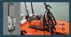
Automatic lifter avoids accidental loosening or bumping. Auto winch to deploy SVP/CTD for profile surveying.
