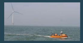
Hybrid propulsion supports operations of up to 24 hours; Unmanned work mode reduces carbon emission.
