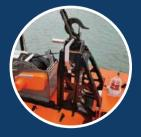
Smart auto-winch structure supports equipment tow service and foldable lifter protect the wet-ends of the sensors.
