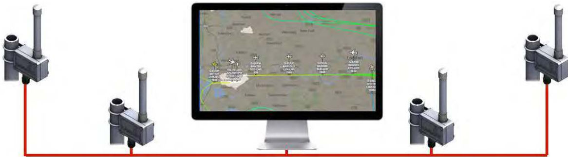
Figure 11: Multiple PingStations may be networked together to provide a wide area low-altitude RID and surveillance volume.
