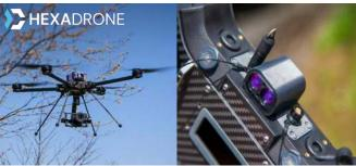
Hexadrone SAS, a French company specializing in the mechatronic development of solutions linked to the use of civil and military drones, equips its multi-functional, modular drone called Tundra with a Fischer UltiMate™ USB 2.0 connector that is waterproof, reliable in all conditions and suitable for intensive use in the field.
