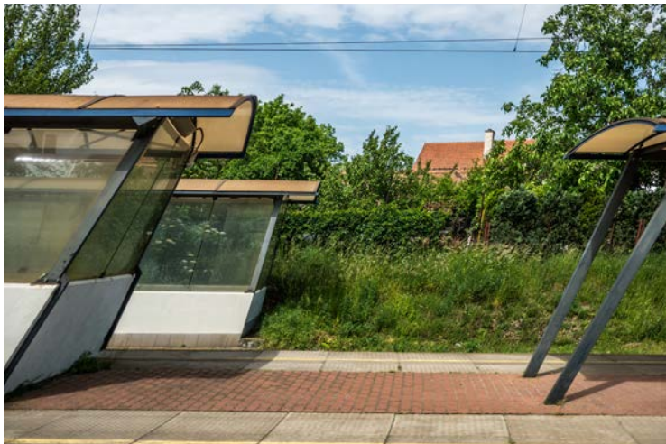
Figure 2 – Image with Skew Caused by a Sensor With a Rolling Shutter
