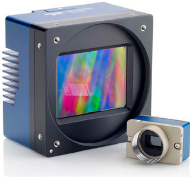
Figure 10: Size contrast between a smaller Genie Nano 1GigE camera and a Falcon4 86M.
