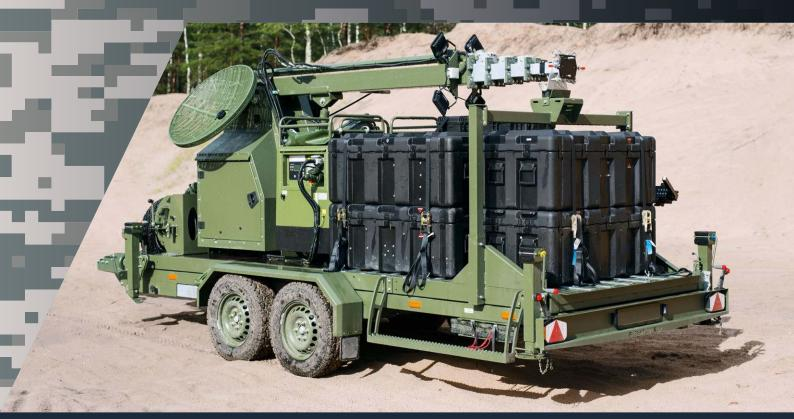
All terrain trailer with hydraulic 15 meter mast. Advanced tracking antenna system with automatic calibration, digital MIMO datalink system and MESH networking. Integrated Power Generator, UPS and cargo platform for transporting Unmanned Aircraft Systems (UAS).
