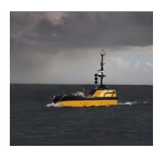
C-Worker 7 is a robust, offshore workclass designed for inspection and positioning applications, C-Worker 7 can negate the need for a ship on station or seabed anchoring.
