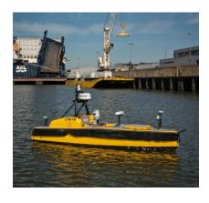
C-Worker 5 is an autonomous vehicle designed to support hydrographic survey work and to increase survey coverage in limited timeframes. A proven offshore survey "forcemultiplier," C-Worker 5 can operate for up to 8 days at a survey speed of around 5 knots.
