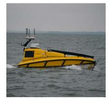
C-Worker 4 is a robust and capable Autonomous Surface Vehicle (ASV) ideally suited to inshore and coastal survey work.
