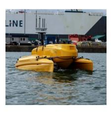
The C-Cat 3 Autonomous Surface Vehicle (ASV) is a rapidly deployable catamaran ideally suited to shallow water operations in inshore and coastal environments.
