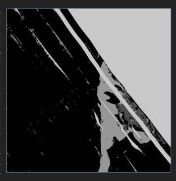
The result of the Seabed Classification module is a very accurate geo-referenced mosaic of seabed types. This mosaic can also highlight regions of the seabed that have not been measured by the survey.
