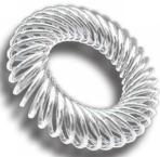
The solutions we develop begin with proven Bal Seal Canted Coil Spring<sup>®</sup> technology. In electrical conducting and EMI/RFI shielding applications, the spring's individual coils provide multi-point contact, and they compensate for mating surface irregularities and misalignment. As a contact component, the spring offers superior conductivity and power density. It runs cooler than other contact technologies, and it is also self-cleaning.
