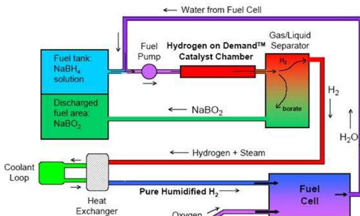
Figure 6: Sodium borohydride system flow diagram
