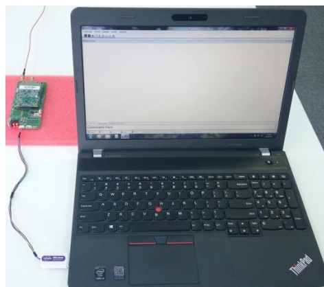
Figure 2 Connect Precis-BX305, Tersus USB Connector and PC
