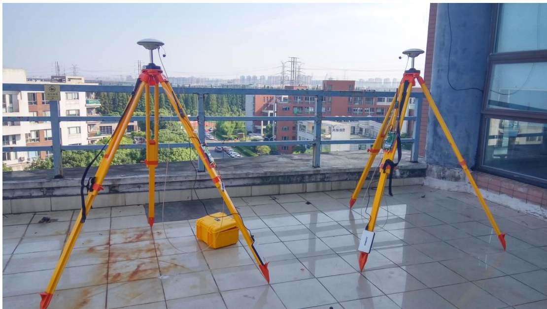
Figure 6 Set up Base and Rover Stations
