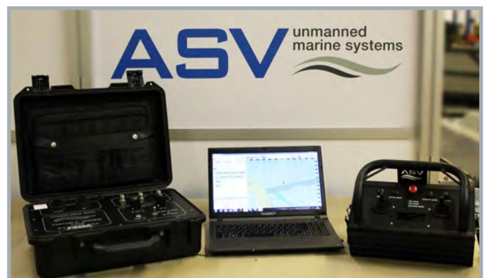
ASView+ control console, software and belly pack.
