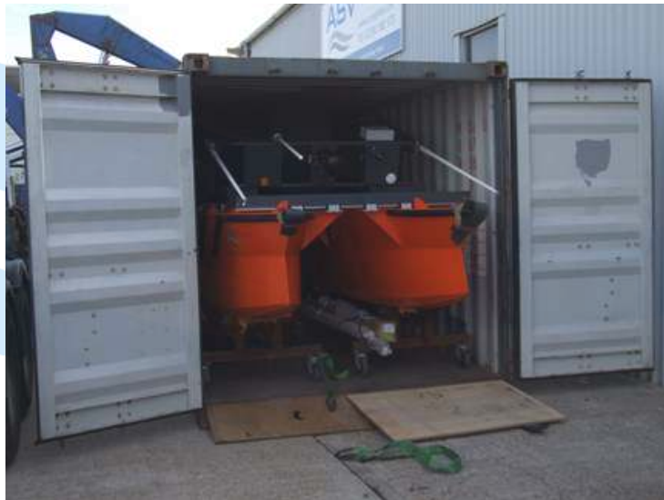
Systems folds for transport in standard 20' container
