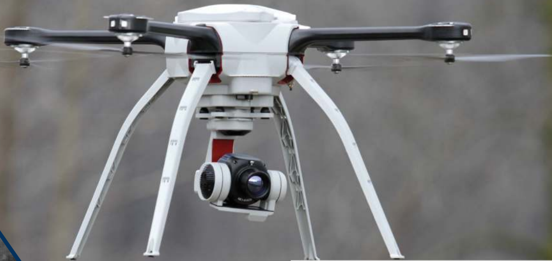
Keii MC-1 Thermal Imaging Payload
